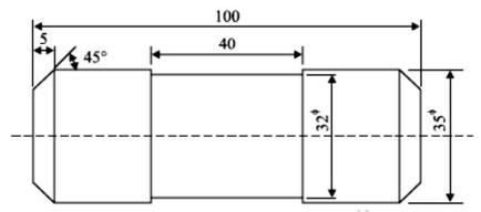
Solution : Ist operation : Turning from f 38 mm to f 35 mm
