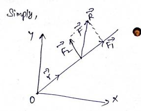
Mo =  $\vec{Y} \times \vec{R}$  ::  $\vec{R} = \vec{F}_1 + \vec{F}_2$ =  $\vec{Y} \times (\vec{F}_1 + \vec{F}_2)$ =  $(\vec{Y} \times \vec{F}_1) + (\vec{Y} \times \vec{F}_2)$ Mo =  $\vec{Y} \times \vec{R} = (\vec{Y} \times \vec{F}_1) + (\vec{Y} \times \vec{F}_2)$ .: Hence, theorem prooved, Rectangular Components of the moment of force.
