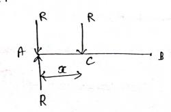
Apply for R' at point A both in the upward and downward directions. (There was no charge in system by this apply).
