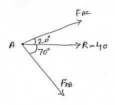
The truck is to be towed using two ropes, Determine the magnitudes of forces frand for acting on each rope in order to develop a resultent force of 950N directed along the positive X-axis.
