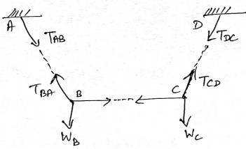
Ex: A electric light fixture weighing 150 N hongs from a point c, by two strings Ac and Bc shown in diagram: Determine the forces in the strings AC and Bc.
