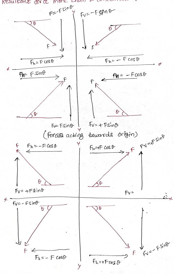
Three Coplanar concurrent forces are acting at a point as given oliggram. Determine the resultant in magnitude and direction.
