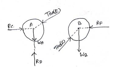
A String APCD, attached to two fixed points A and D has two equal weights & loop N attached to it at B and C. The weight rost with the portions AB and CD inclined at angles of 30° and 60° respectively, to the vertical as given in diagram. Find the bensions in the portions AB, BC, CD at the String, the inclination of the portion BC with the vertical is 120°.
