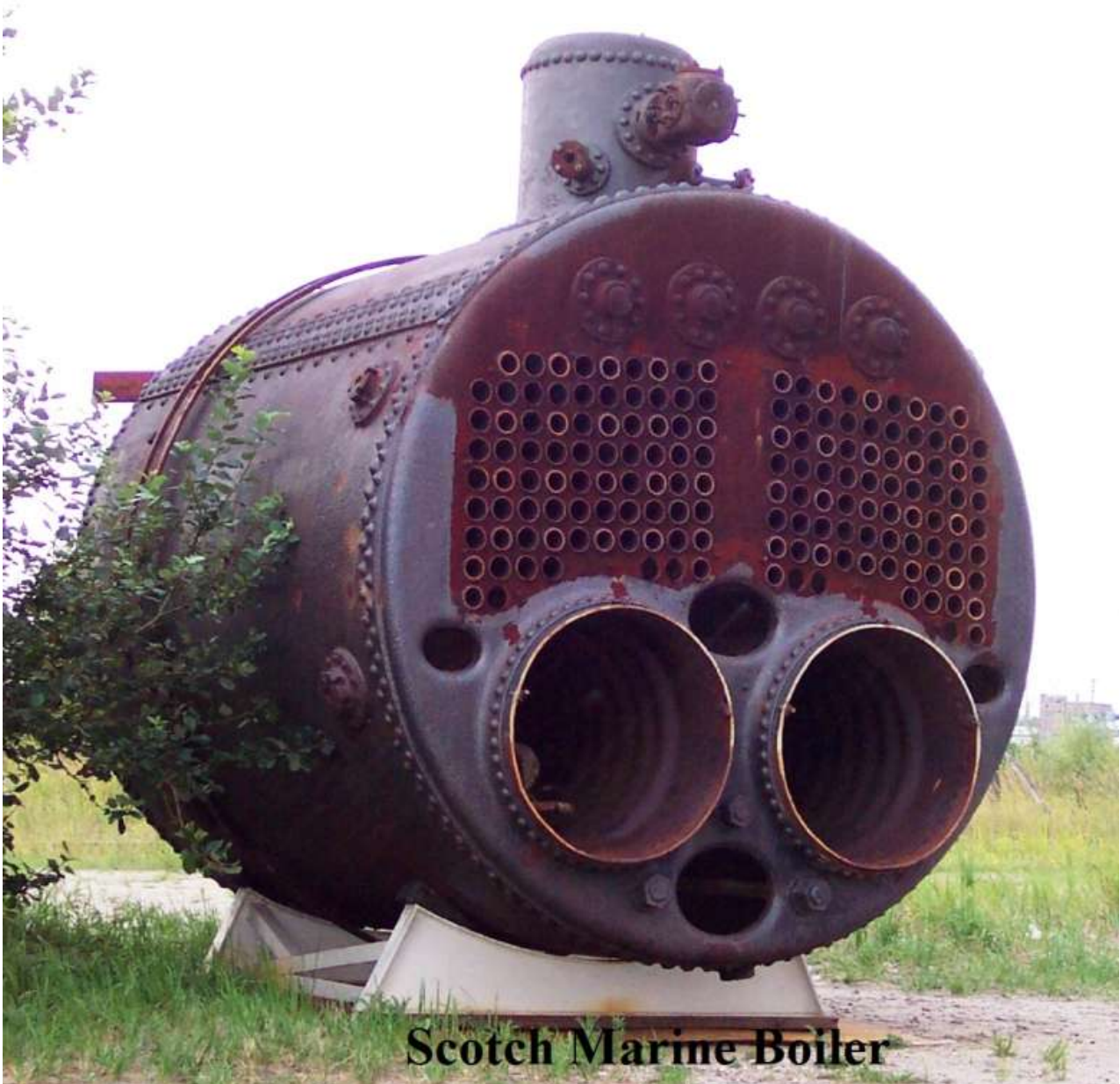
Scotch marine boiler
