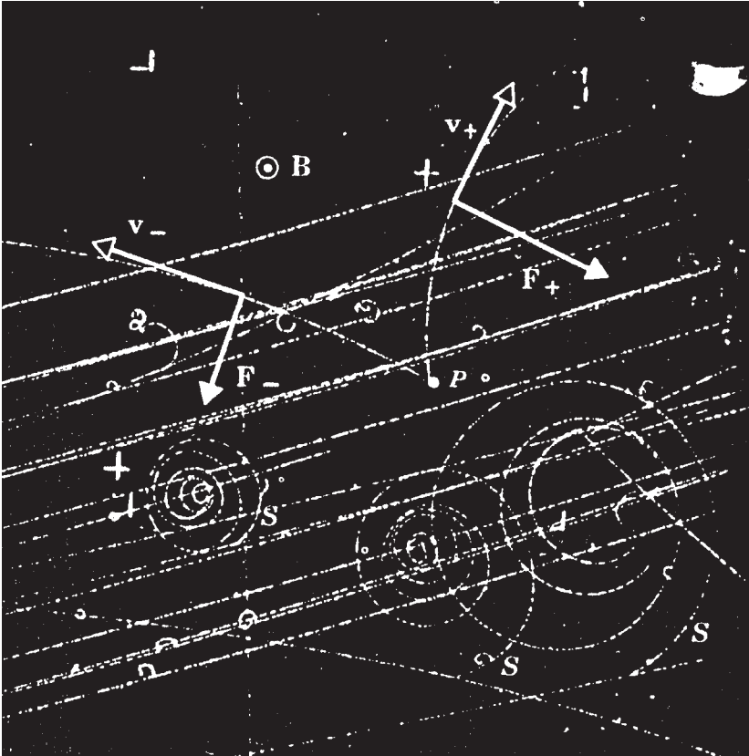
FIGURE 26.6 A bubble chamber is a device for rendering visible, by means of small bubbles, the tracks of charged particles that pass through the chamber. The figure is a photograph taken with such a chamber immersed in a magnetic field B and exposed to radiations from a large cyclotron-like accelerator. The curved V at point P is formed by a positive and a negative electron, which deflect in opposite directions in the magnetic field. The spirals S are tracks of three low-energy electrons.
