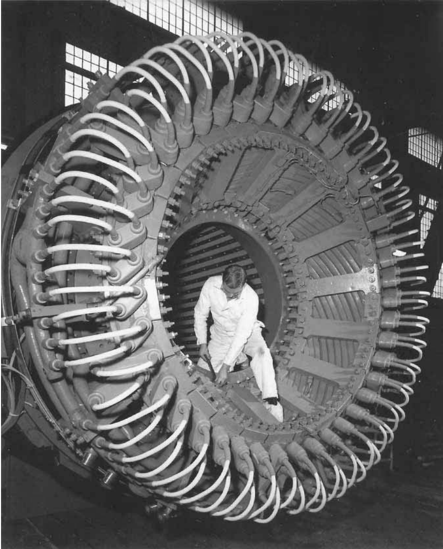
FIGURE 32.24 View of a 660-MW generator stator end windings.
