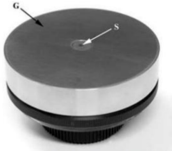
Figure 3.8 Hand-grinding jig for TEM specimen preparation. A disc (S) is glued to the center of the jig and the guide ring (G) controls the amount of grinding.
