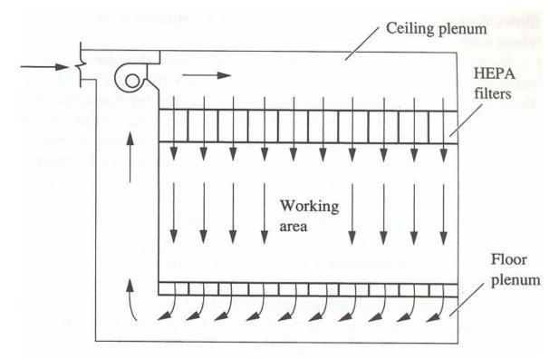
Fig.39.12(a): Downward unidirectional flow
