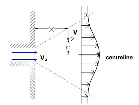
Fig.39.4: Velocity distribution through a circular jet
