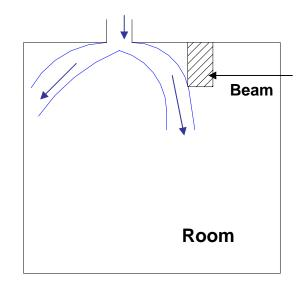
Fig.39.1(a): Drop of a cool air jet
