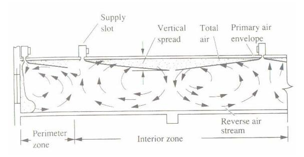
Fig.39.11: Airflow pattern for cooling using slot diffusers
