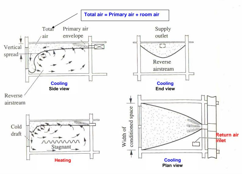
Fig.39.9: Airflow pattern using high side outlets for cooling and heating applications
