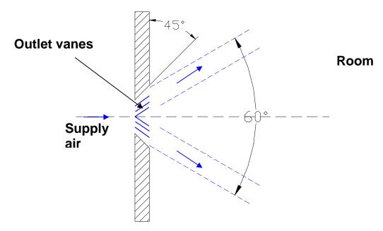
Fig.39.3: Spread of an air jet with diverging vanes
