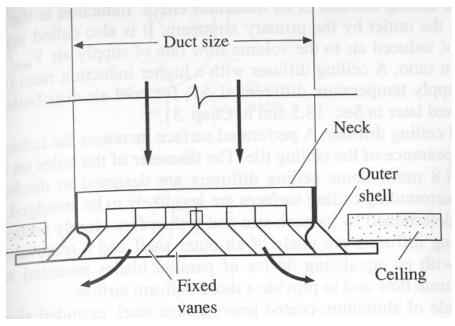
Fig.39.6(a): Schematic of a ceiling diffuser
