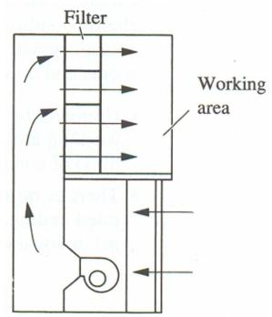
Fig.39.12(b): Horizontal unidirectional flow
