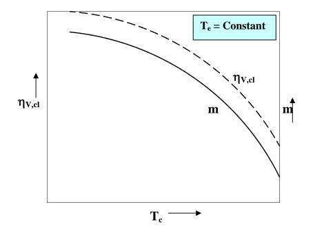
Fig.19.6. Effect of condenser temperature on clearance volumetric efficiency and mass flow rate of refrigerant
