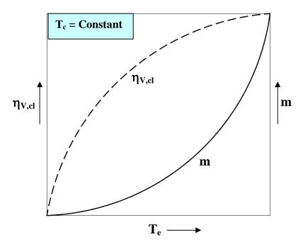
Fig.19.2. Effect of evaporator temperature on clearance volumetric efficiency and refrigerant mass flow rate
