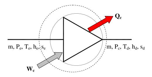
Fig.18.3. Energy balance across a steady flow compressor
