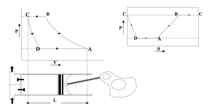
Fig.18.4. Ideal reciprocating compressor with clearance
