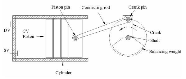
Fig 18.1: Schematic of a reciprocating compressor
