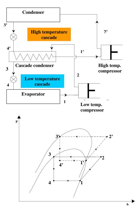
Fig.13.6(a) & (b): A two-stage cascade refrigeration system
