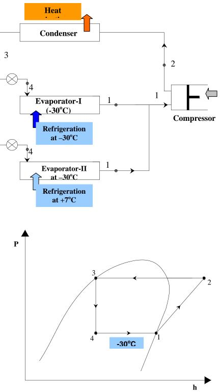
Fig.13.1(a) & (b): A single stage system with two evaporators
