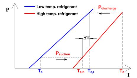
Fig.13.7(b): Schematic illustrating principle of two-stage autocascade system on D<sup>°</sup>hring plot Version 1 ME, IIT Kharagpur 16
