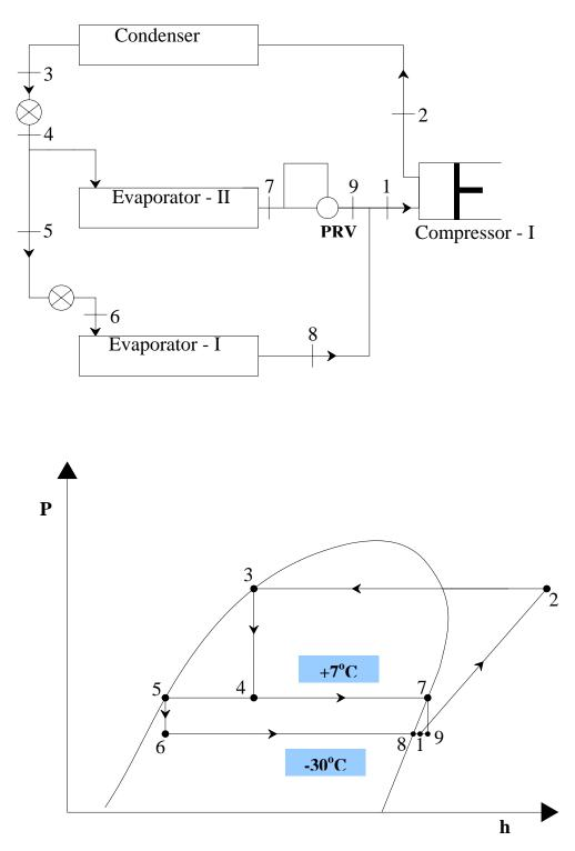
*Fig.13.3(a) & (b): Multi-evaporator system with single compressor and multiple expansion valves*
