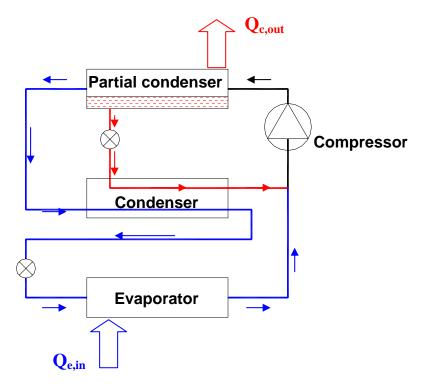
Fig.13.7(a): Schematic of a two-stage auto-cascade system
