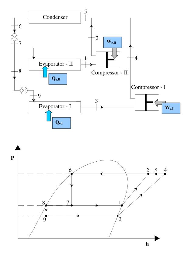
Fig.13.5(a) & (b): Multi-evaporator system with individual compressors and multiple expansion valves
