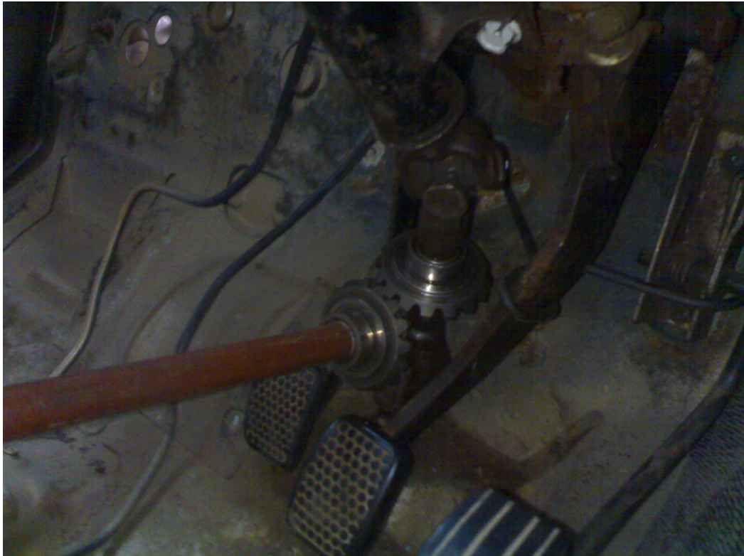
Fig 9.3 Bevel Gear Arrangement with Front Steering System
