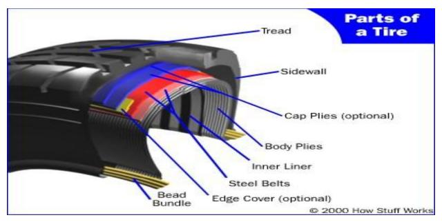
As illustrated below, a tire is made up of several different components.
