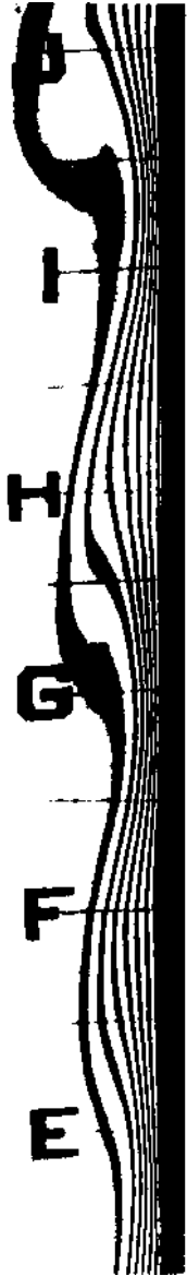
Figure 7-3 | Pulsed free-convection boundary layer on vertical flat plate. Distance between letters = 5 cm.
