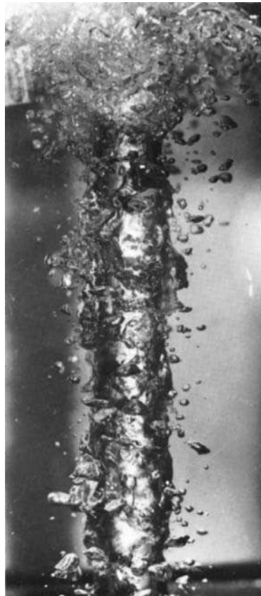
Figure 9-7 | A steam-heated vertical 19.05-mm-diameter copper tube displaying turbulent film boiling in methanol. \Delta T_x = 138^\circ\text{C} q/A = 38.8 \text{ kW/m}^2 .
