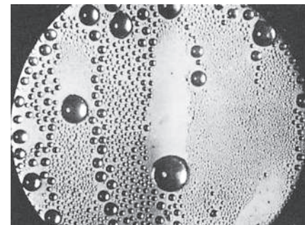
FIGURE 10-35 Dropwise condensation of steam on a vertical surface (from Hampson and Özişik, Ref. 11).
