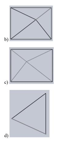
*Explanation:* The isometric view should be drawn according to the given views and in such a way that maximum possible details are visible. Arrow mark in the given figure show the direction in which front is taking and dotted lines represent hidden edges and lines.
