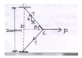
15.Two cables are tied together at c and are loaded as shown in fig below. Determine the tension in the cable AC and BC
