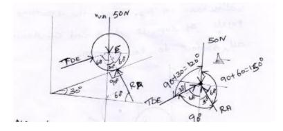
No of forces is three, apply Lami's Theorem
