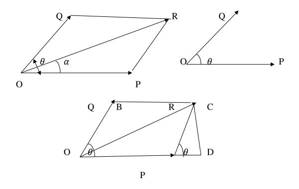
Let pand Q are two concurrent force acting on a point O at an angle of  $\theta$ .
