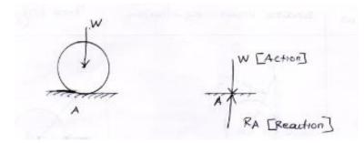
Consider a Ball placed on a horizontal surface shown in fig. The self weight of the ball (w) is acting vertically downwards through its centre of gravity. This force is called Action.
