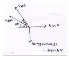
$\Sigma FH = 0 \quad \rightarrow + \quad - \leftarrow$   $450 - T_{AB} \cos 50 - T_{AC} \cos 30 = 0$   $T_{AB} \cos 50 + T_{AC} \cos 30 = 450$   $0.64T_{AB} + 0.86T_{AC} = 450 - \dots (1)$
