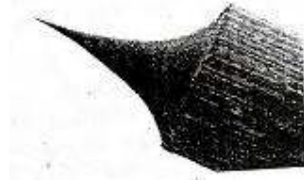
Fig. 6.17 Tungsten tip of STM
