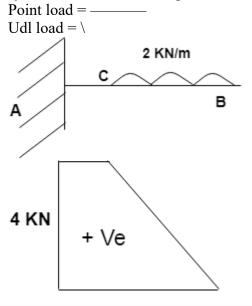
7. \_\_\_\_\_ curve is formed due to bending of over hanging beams.
