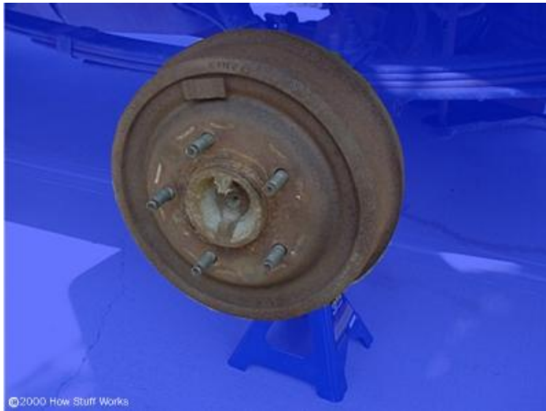
Figure 2. Drum brake with drum in place
