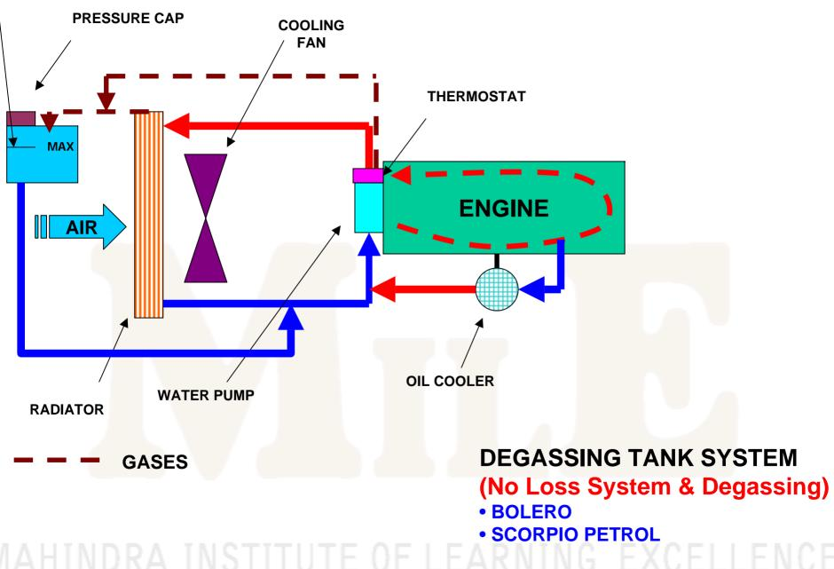
**1. WATER PUMP** - Water pump sucks water from the radiator bottom tank and pushes the water in to the engine block/cylinder head. Water pump is driven by the engine crankshaft by a belt (in some cases it may be gear driven)
