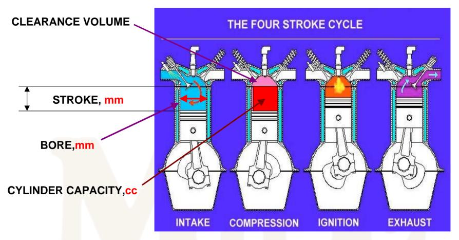
ENGINE CAPACITY, cc = CYL. CAPACITY X No OF CYL UNITS - cc - Cubic centimeter - Lit - Liters = cc/1000
