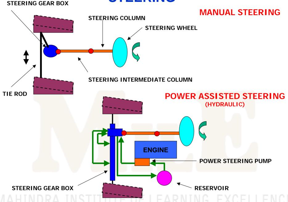
1. STEERING GEAR BOX - Steering gear box converts driver's effort at steering wheel (Rotary) to a linear movement at tie rods. The tie rods are connected to the wheels which turn either left or right.
