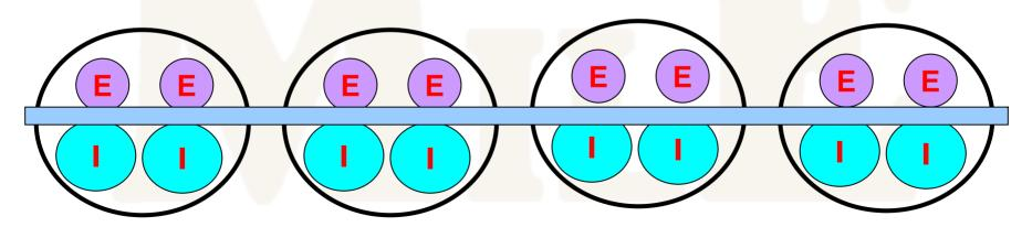
**4 VALVES/CYL , SOHC - VALVES OPERATED THROUGH ROCKERS**
