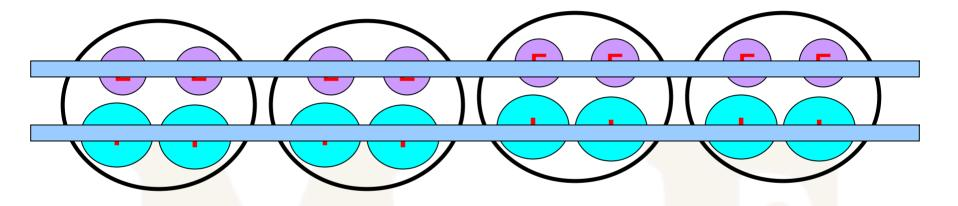
**4 VALVES/CYL , DOHC - VALVES OPERATED EITHER DIRECTLY OR THROUGH ROCKERS**
