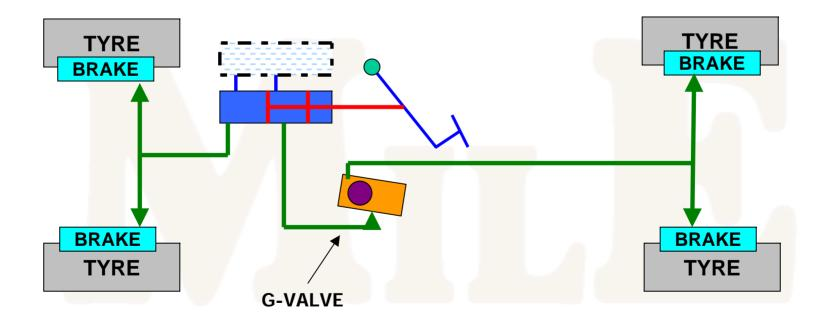
G-Valves are fitted at a specified angle in direction of vehicle motion
