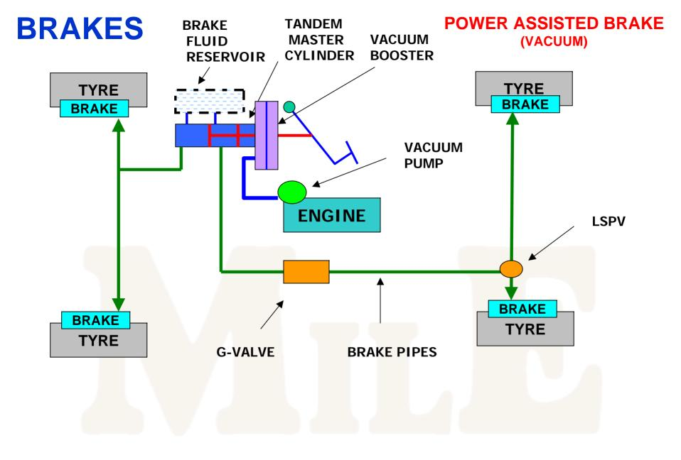
**1. TANDEM MASTER CYLINDER** - Converts driver's foot effort to hydraulic pressure and transmits the pressure to wheel cylinders.
