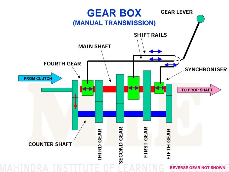
**GEAR RATIO** - Gear ratios are gear reduction steps in the gear box. A gear reduction multiplies the engine torque by the gear ratio amount. Torque requirement at the wheel depends operating conditions. For example :
