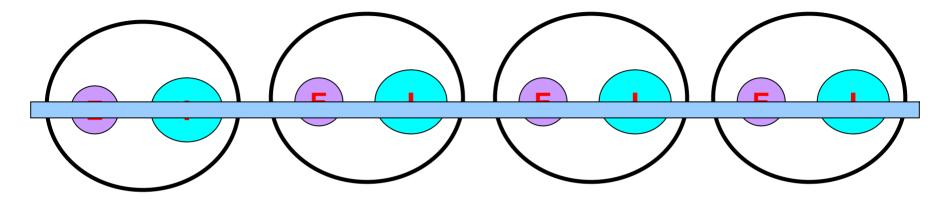
2 VALVES/CYL , SOHC - VALVES OPERATED EITHER DIRECTLY OR THROUGH ROCKERS
