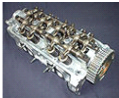
A single overhead camshaft (SOHC) cylinder head from a Honda D15A3
