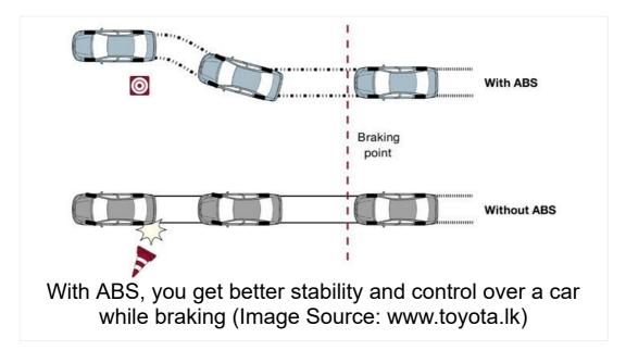
A skidding wheel (where the tire contact patch is sliding relative to the road) has less traction (grip of the tire on the road) than a non-skidding wheel. For example, if your car drives over a road covered in ice, it is unable to move forward and the wheels will keep spinning, since no traction is present. This is because the contact point of the wheel is sliding relative to the ice.
